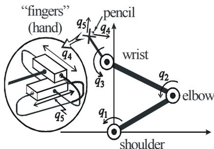
**Figure 1.** Mechanism configuration with five DOF
