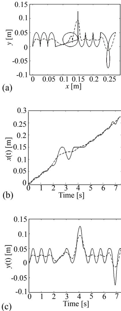
**Figure 3.** Definition of the task: (a) sequence of letters; (b), (c) time histories of operational coordinates. The solid lines show the prescribed motion, and the dashed lines show the smooth components
