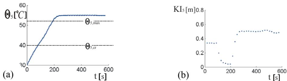
**Figure 6.** Behavior of joint No. 5: (a) joint fatigue  $\Theta_5(t)$ , (b) joint involvement  $KI_5(t)$ .
