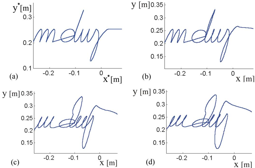
**Figure 8.** Gradual degeneration of writing. (a) Reference sequence. (b)-(d) Degenerated sequences are recorded for the following repetitions: (b) 12<sup>th</sup> forward sequence, time:  $198 \leq t \leq 207$ , (c) 14<sup>th</sup> forward sequence, time:  $234 \leq t \leq 243$ , (d) 22<sup>nd</sup> forward sequence, time:  $378 \leq t \leq 387$ .
