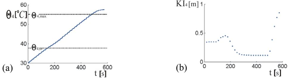
**Figure 5.** Behavior of joint No. 4: (a) joint fatigue  $\Theta_4(t)$ , (b) joint involvement  $KI_4(t)$ .
